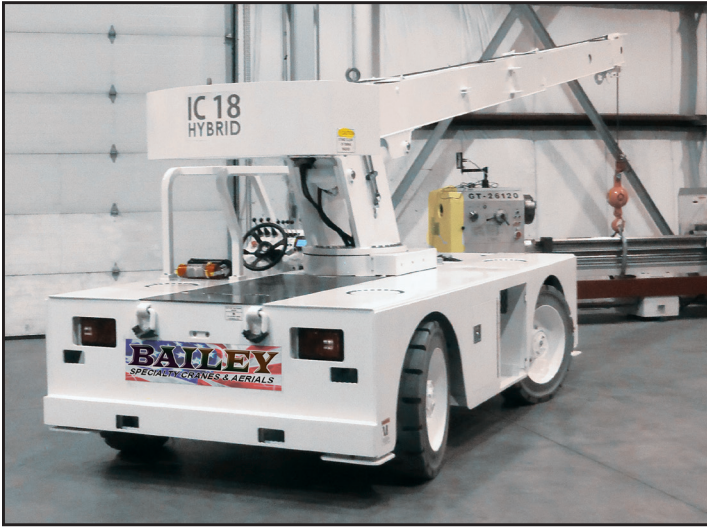
9 Ton Carry Deck Crane
